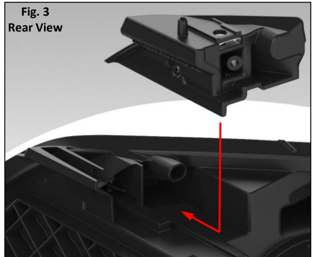
**3. Scuff & Glue:** Scuff the housing and tab(s) using a sanding pad. Remove sanding dust using compressed air. Wipe down the housing and tab(s) using a pre-cleaner to ensure surfaces are free from oil and debris. Apply glue to both the housing and tab(s).
