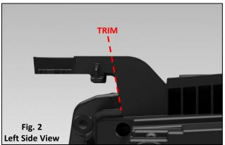
**2. Dry-Fit:** Dry-fit the repair tab(s) **Fig. 3**. If the tab fits without resistance and makes a flush fit to the housing, trimming is complete. If the tab resists installation re-trim the damaged tab, removing only small amounts of material. Repeat the Dry-Fit steps until the proper fit is achieved.
