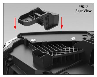
**3. Scuff & Glue:** Scuff the housing and tab(s) using a sanding pad. Remove sanding dust using compressed air. Wipe down the housing and tab(s) using a pre-cleaner to ensure surfaces are free from oil and debris. Apply glue to both the housing and tab(s).
